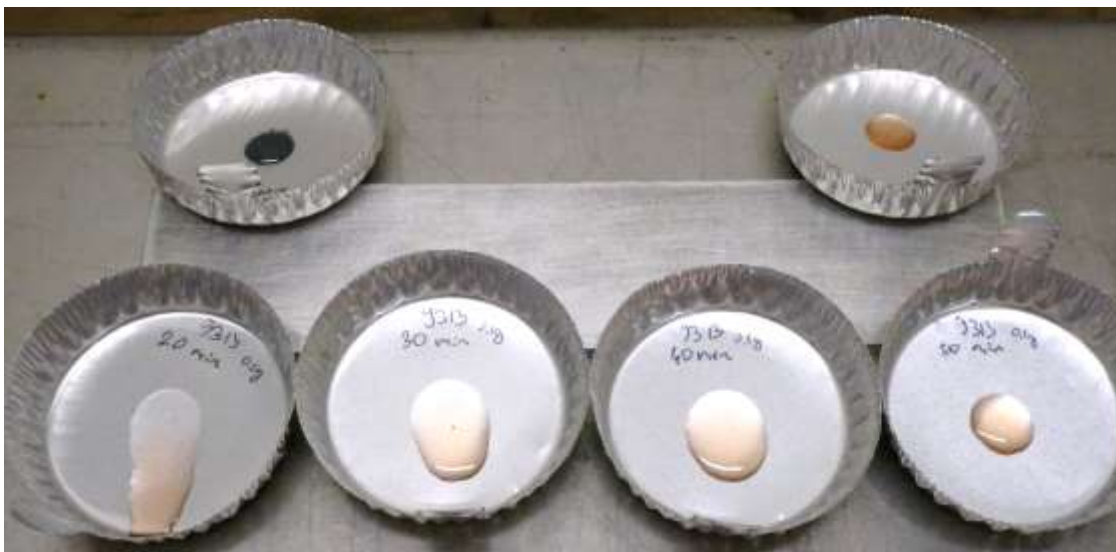
Figure 3. Viscosity Tests: Hysol 9313 at 5 Ten-Minute Intervals (20-60 Minutes Post Mixing), 3M 2216 at 20 Minutes After Mixing
